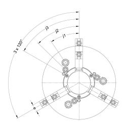
C 15 3-jaw power chucks DURO-A RC, with quick jaw change system, with individual jaw unlocking, with straight teeth, short taper mount DIN ISO 702-1
